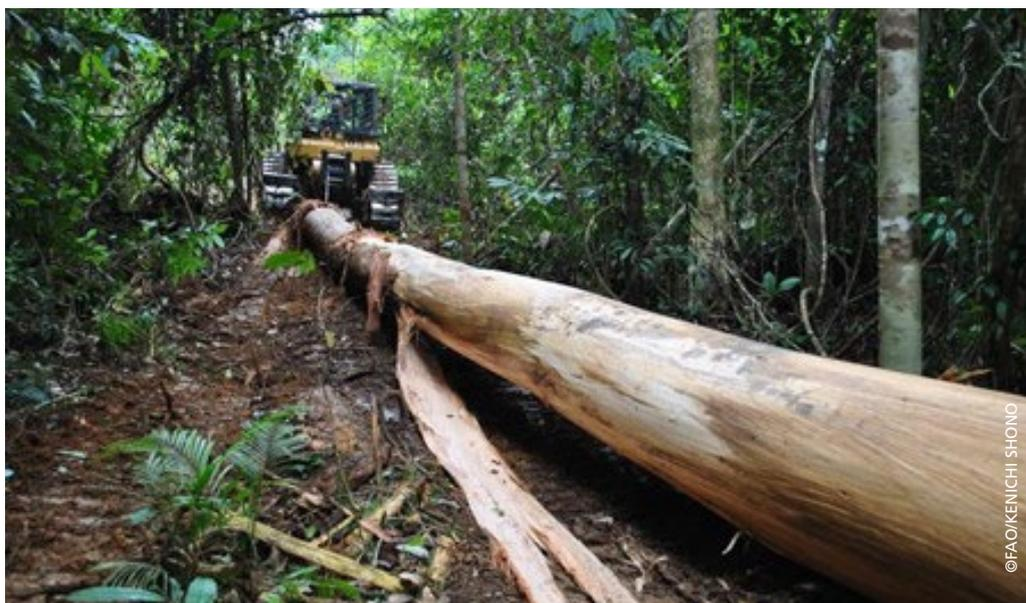
Log extraction with a track skidder in a logging concession in Indonesia
