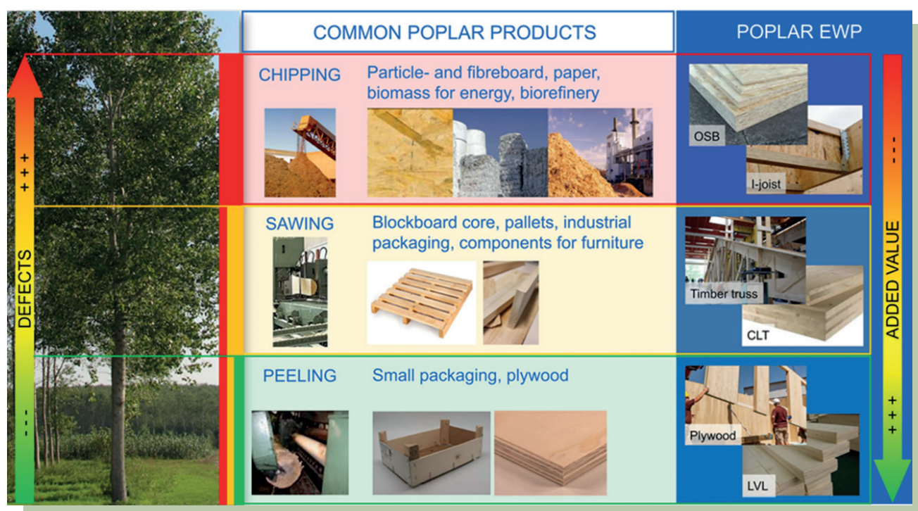
Figure 6. Potential for producing engineered wood products from poplar to complement current poplar-based products in biobased green buildings
